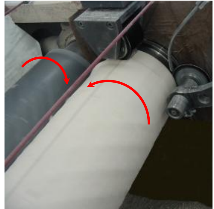
Product felt on front roller
