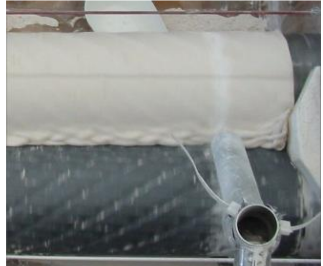
Zone of turbulence at the nip
